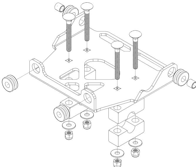
3. Insert the **Y1000** as shown in the diagram, then tighten the **black M6x16 bolts** (maximum torque: **8Nm**), one on each side.
